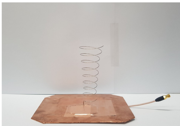
FIGURE 1 Configuration of the proposed SICHA: A, side view; B, perspective view; and C, fabricated antenna. SICHA, stretchable inverted conical helical antenna [Color figure can be viewed at wileyonlinelibrary.com ]
